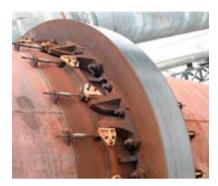
Kiln tyre with tangential suspension
