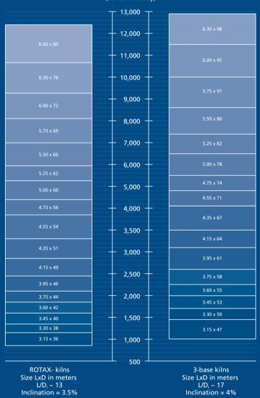
Kiln length is variable within a range and can be designed for special cases. The nominal output is based on normal clinker quality and kiln volumetric loading of 5.0 ton/day/m³ for 3-base kilns and 5.3 ton/day/m³ for ROTAX-2 kiln. The potential output of a kiln also depends on the burnability of the raw materials. The kiln rotational speed is designed for 5.0 rpm (revolutions per minute) with a nominal speed of 3.6.
