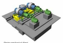
Electro-mechanical direct drive station for ROTAX-2 kiln
