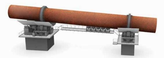
The kiln is the heart of the plant – what an entire cement plant is dimensioned around, and where most of the final chemical reactions take place. So it's not surprising that a producer requires an ideal kiln solution.
