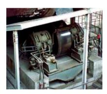
Self-aligning roller support for ROTAX-2 kiln
