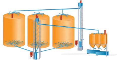
FLSmidth's Airlift™ vertical conveyors and Airslide® gravity conveying systems convey alumina at a net rate of 750 mtph in a major western United States facility
