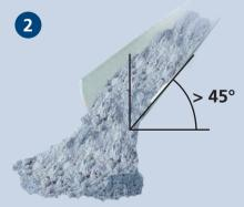
Without any fluidization, the Airslide® conveyor would need to be inclined on an angle greater than the angle of repose to establish gravity flow.
