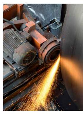
Thrust face grinding
