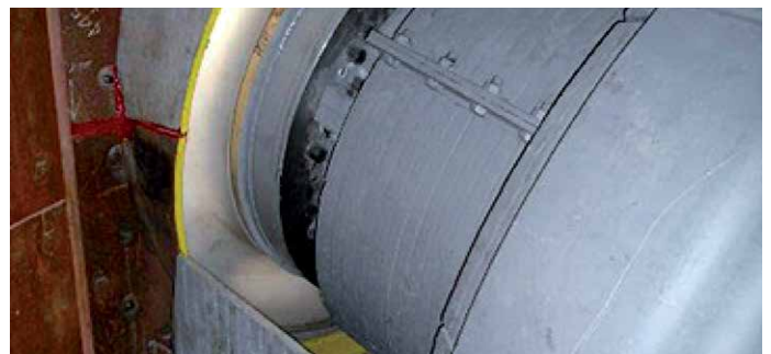
Flexible seal between housing and roller
