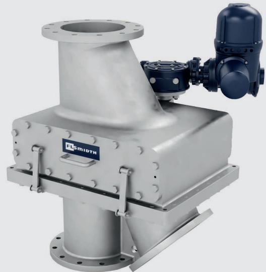
The SK V2 two-way valve is available in five sizes: 150mm (6"), 200mm (8"), 250mm (10"), 300mm (12") and 350mm (14") and matches the I.d. of standard schedule 30 pipe. Flanges are available in ANSI or DIN designs, with 45° divert port as standard.
