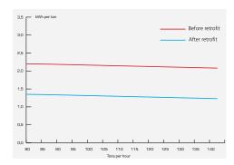
The diagram exemplifies the difference in power consumption before and after a retrofit
