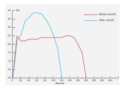
The diagram exemplifies the difference in dispatch time before and after a retrofit. The level of the curves indicates pump pressure during dispatch of a batch of cement.
