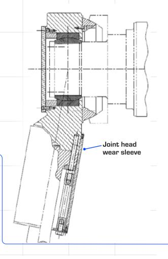
Split wear sleeves eliminate much of this complexity. They can be replaced simply by removing the joining bolts without disturbing the joint head and pull rod fixing bolts, cutting the time needed for sleeve maintenance. The split design is now supplied as standard for ATOX® mills.
