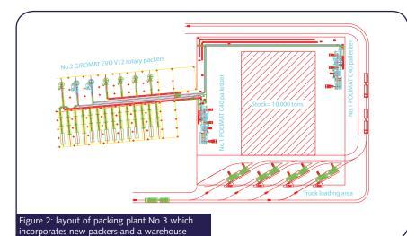
loaded onto trucks by forklift. This results in fast, efficient dispatch. Several trucks can be loaded simultaneously and different types of products can be loaded onto the same truck. The use of slip sheets means stacks can be loaded onto a truck's own pallet, thereby simplifying logistics and avoiding empty pallet costs.
