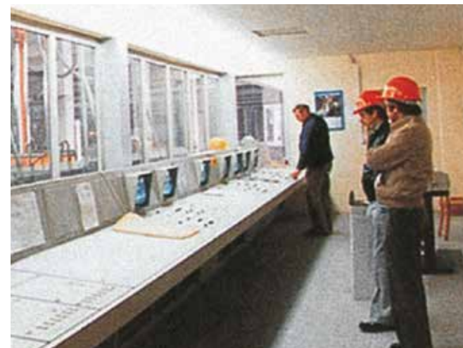
One operator in the control room managing more CARICAMAT automatic truck loaders.
