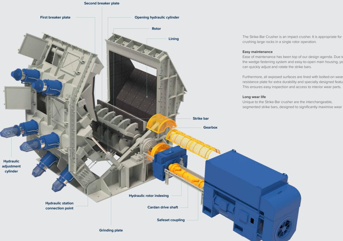
Ease of maintenance has been top of our design agenda. Due to the wedge fastening system and easy-to-open main housing, you
