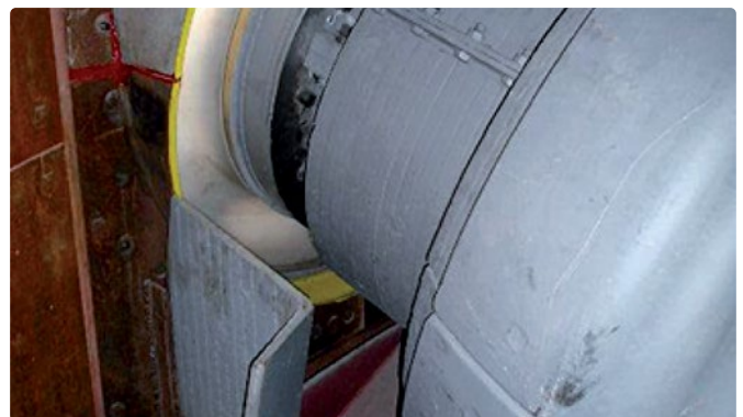
Flexible seal between housing and roller
