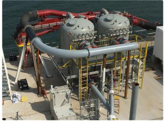
Starting with a range of four basic sizes, FLSmidth Cement can supply the right DOCKSIDER ship unloader for any terminal – whether you're unloading river barges or Handymax bulk vessels, and whether you're conveying to an adjacent belt conveyor or through a 1200 m (4000 ft) pipeline.
