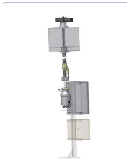
Airslide spot sampler (shown with optional local control cabinet)
