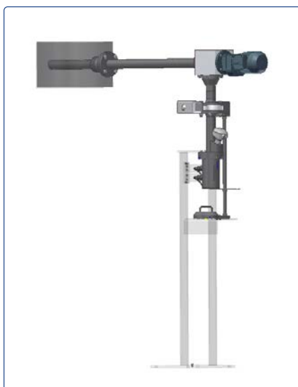
Screw spot sampler in ATEX execution for sampling of coal meal.
