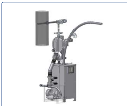
Screw+mixer composite sampling station with excess sample material return blower.
