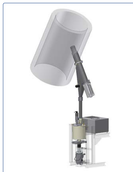
Hot meal spot sampler including water cooling device for fast cooling of sample.
