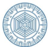
Figure 3: 7-compartment CFMI silo
