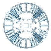
Figure 2: CFMI silo with 4 equally sized compartments
