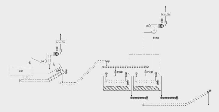
Typical flow diagram for processed alternative fuel storage and feed
