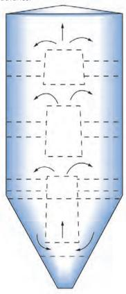
The column blender can accommodate different volumetric batch sizes.
