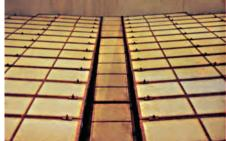
Top: complete coverage for maximum fluidizing effect; Bottom: center or side withdrawal - all material flows toward center trough
