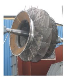
Impeller, delivered pre-assembled
