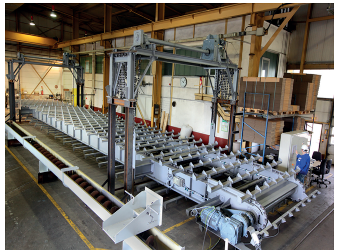
Feedex™ overhead reclaimer
