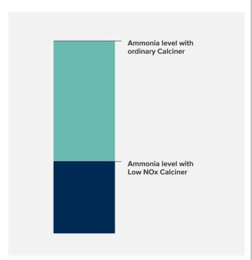
In many cases, our Low NOx Calciner will be sufficient to meet NOx targets without the use of NOx reduction systems. If ammonia is still needed, the amount of ammonia is reduced.
