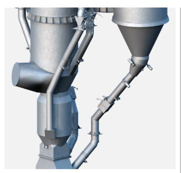
For optimal NOx reduction and minimised wall build-ups, the reduction zone has a round design with two raw meal inlets.
