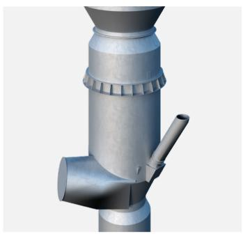
The unique design of the lower calciner optimises dispersion of the raw meal into the gas stream.
