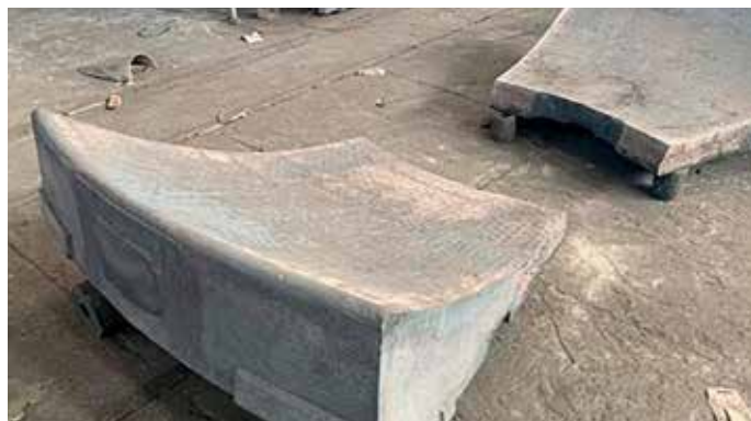
OK™ Pro+ wear liners are currently available for rollers and tables of all OK™ raw mills and most OK cement mills with full roller segments.
